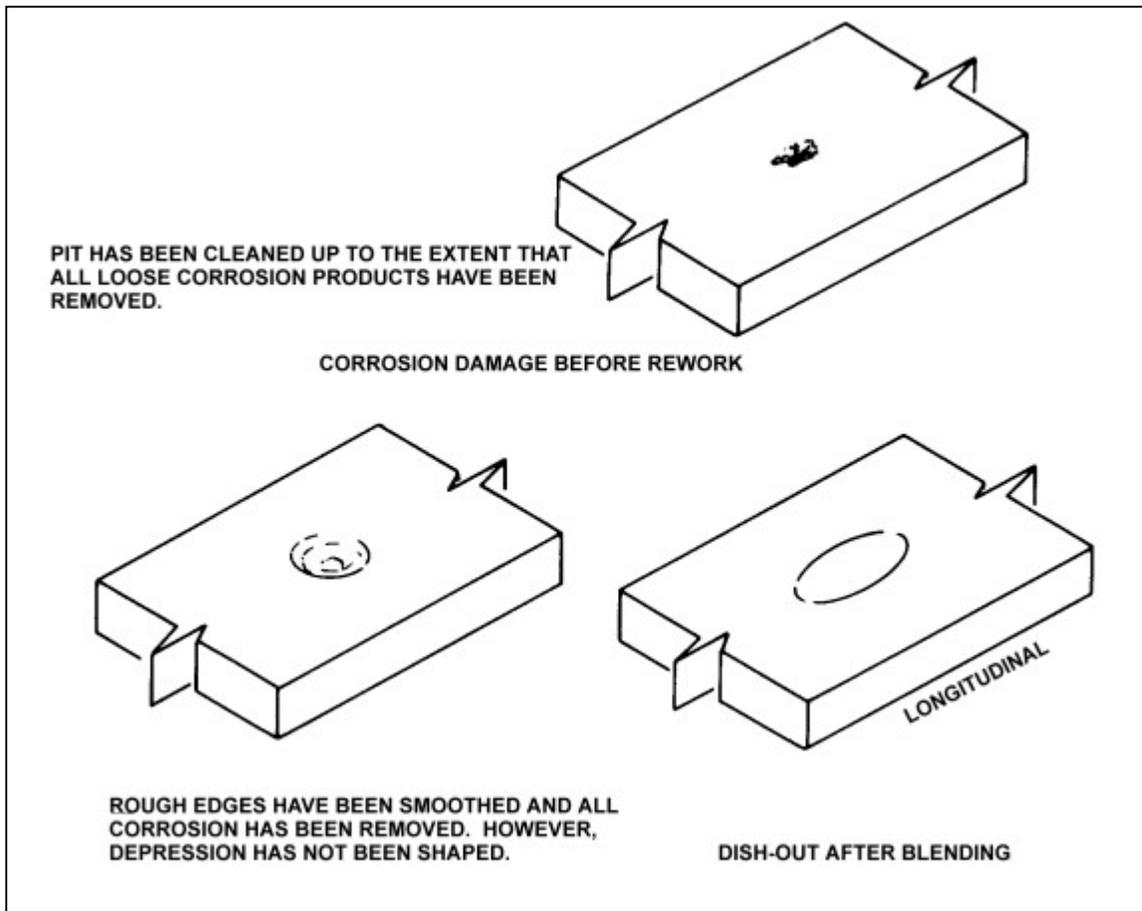
FIGURE 6-15. Blendout of corrosion as a single depression.
